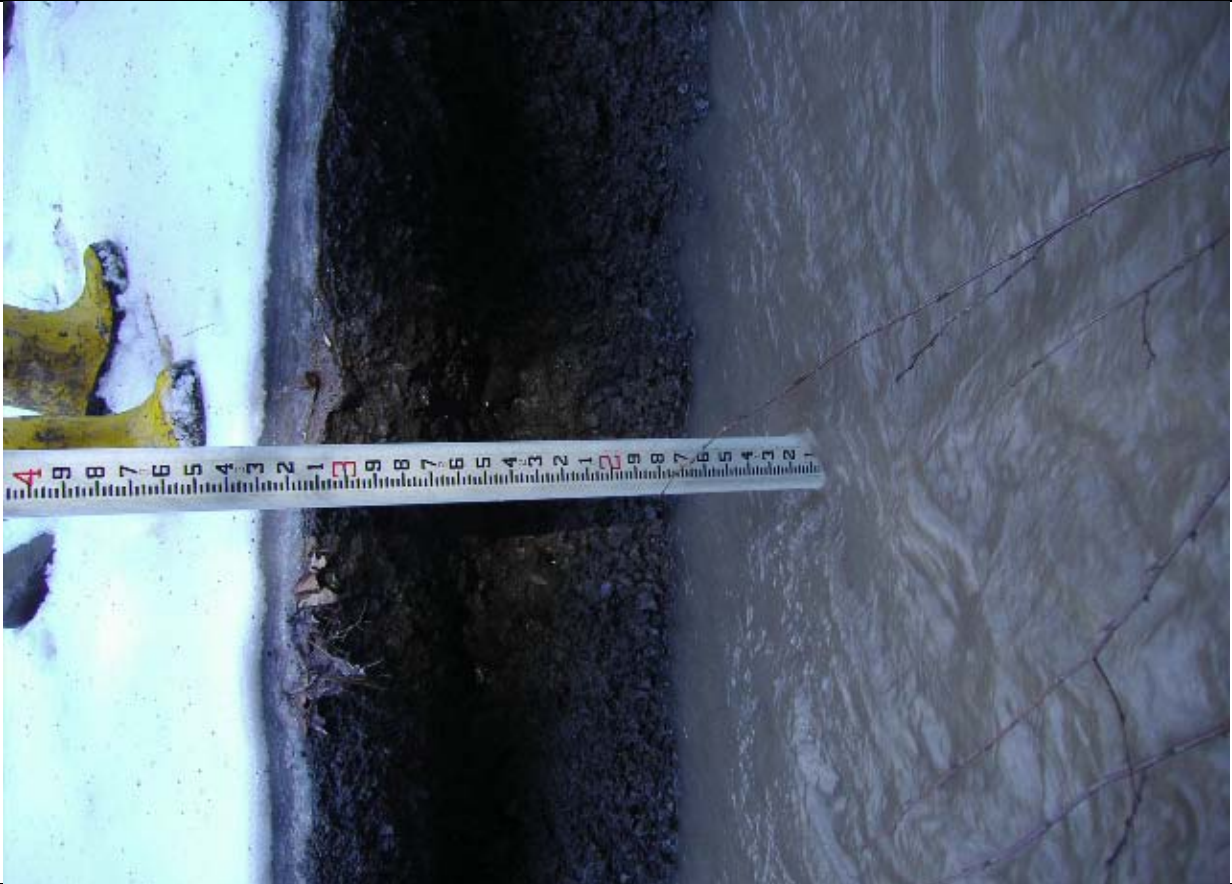
Photo 173 (3/08/12): R. bank just downstream of photo 55 showing 3+-ft of downcutting
