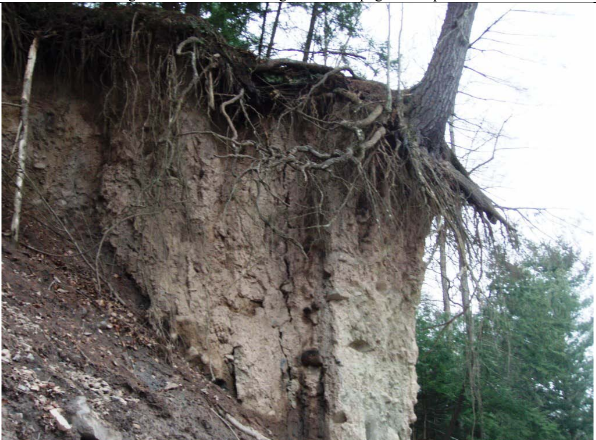
Photo 15: close-up of white pine on failed left bank with failure plane crack visible
